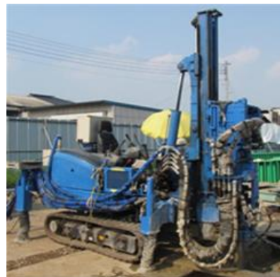
Figure 1. Construction machine for soil-cement composite piles.
