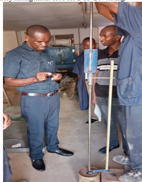
Figure 2. Laboratory DCP-DN set up
