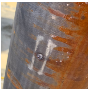
Figure 6. Test Zillertal: Sheared screw that held an accelerometer.
