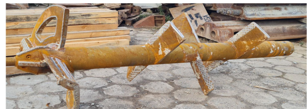
Figure 5. Deep soil mixing tool
