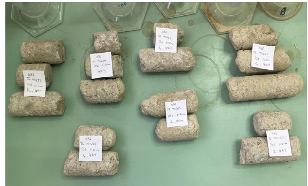
Figure 10. Core samples from a DSM test column
