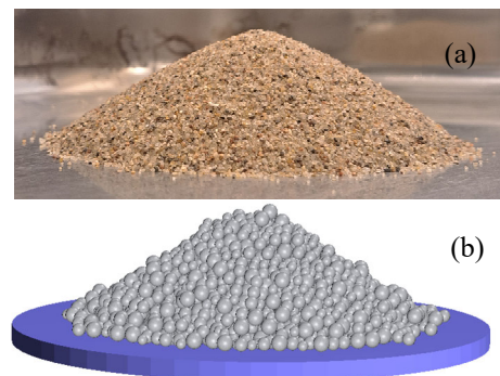
Figure 1. Comparison between physical (a) and numerical (b) angle of repose
