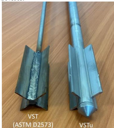
Figure 4. Photograph of the VSTu apparatus and comparison with the conventional VST apparatus (ASTM D2573).
