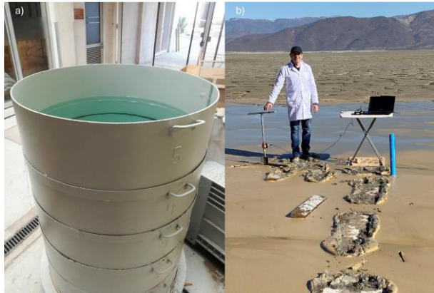
Figure 3. a) 1 m diameter container for VSTu test. b) Field VSTu test on tailings impoundment, near the water pond.
