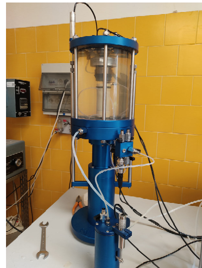
Figure 2. The cyclic Bishop and Wesley triaxial cell of geotechnical laboratory of University of Naples Federico II (Italy).
