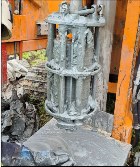
Figure 1. Quick clay sample collected from a depth of 8,2 meters at the NGTS site.
