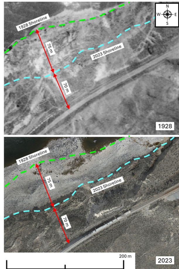
Figure 3. Progressive shoreline erosion between 1928 (top) and 2023 (bottom).
