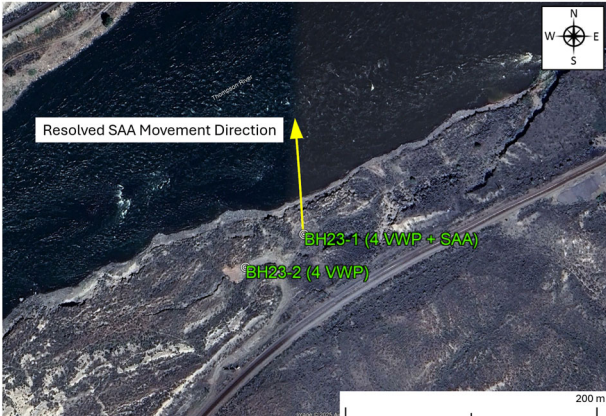
Figure 8. Clifton borehole investigation layout in 2023.
