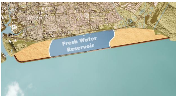
Figure 1. Coastal reservoir as part of an integrated solution for sea level rise
