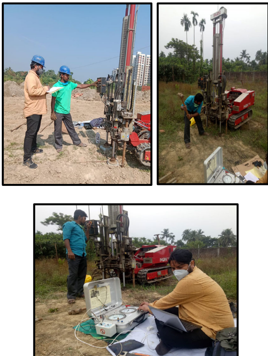
Figure 2. CPT, SDMT, and DMT tests being carried out during the in-situ test campaign at the study area.
