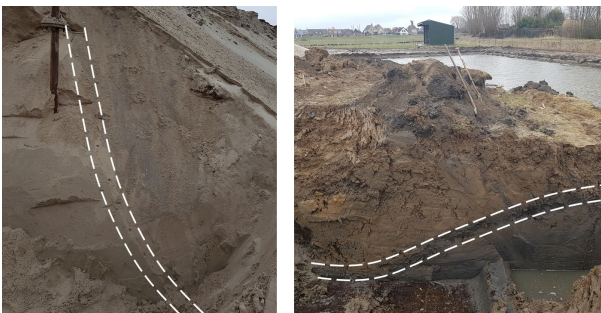
Figure 10. Left: Failure surface at the embankment in the sand layer 1a indicated by the dashed lines. Right: failure surface at the toe in soft clay layer 3a just above peat layer 4 (Lengkeek, 2022).
