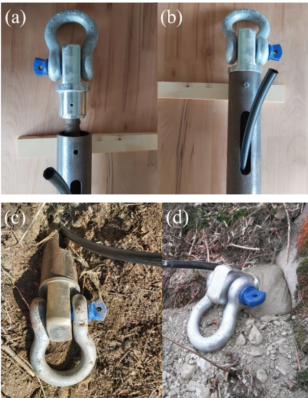
Figure 2. Rigid connection between pile head and pipe reinforcement (a, b) and built-in pile head system in alpine terrain (c, d).
