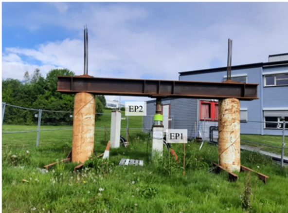
Figure 1. Test Setup: Energy piles with reaction beam on the main pile
