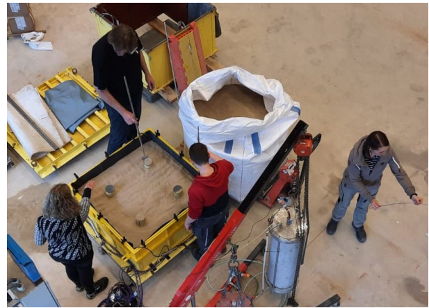
Figure 1. Building the small scale model prior to testing, including four piles with a diameter of 0.1 m (2022, Deltares Geo Model Hall facility)
