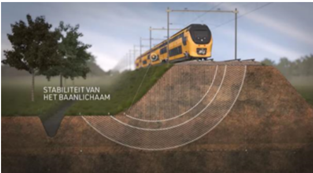
Figure 2. Example of sliding plain in the track embankment
