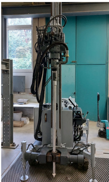
Figure 5. Modified drilling rig for screwing in small-scale drilling tools.
