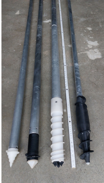
Figure 4. Small-scale full displacement bored pile tools on a scale of 1:10: from left to right: Fundex ( \varnothing 40/56 mm), Atlas ( \varnothing 45/62 mm), Quast-VVB ( \varnothing 60 mm), Jac-V ( \varnothing 60 mm).
