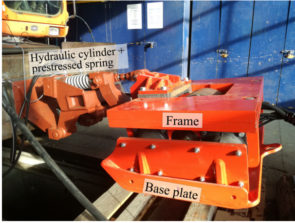
Figure 2. Plate compactor attached to an excavator (Sigmund, Pistol and Adam, 2023).
