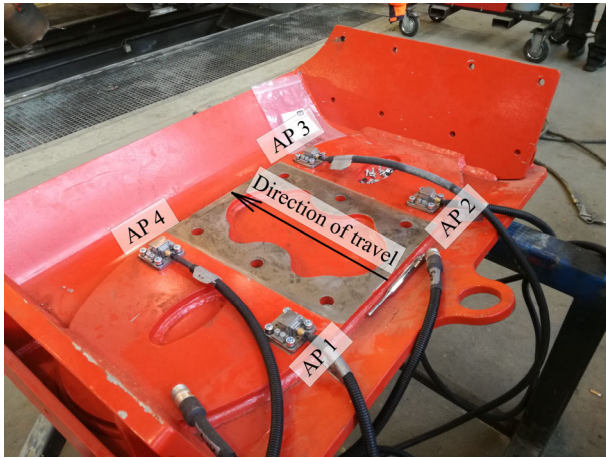
Figure 3. Base plate equipped with acceleration sensors.
