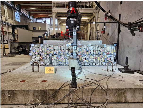
Figure 4. Test set-up. A=vertical actuator used to apply the vertical load N ; t=displacement transducers used to measure the vertical displacement \delta_v .
