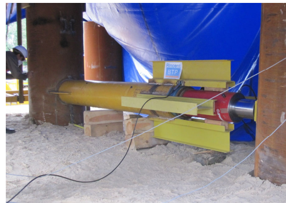
Figure 9. Lateral test using 2 piles, one acting as reaction
