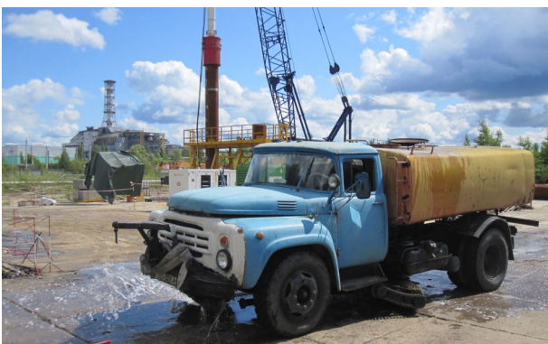
Figure 4. Watering device for soil decontamination in remote areas
