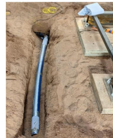
Figure 5. Image of the instrumented pipe in the trench.
