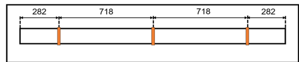
Figure 4. Position of circumferential OBR4600 optical fibres on test duct (dimensions in mm).
