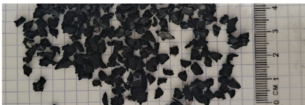
Figure 7. Rubber crumbs used for the subsoil composite layer.
