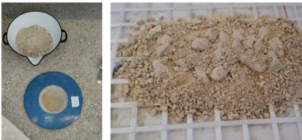
Figure 6. Left: Subballast layer made of gravel (photo taken during density determination by sand replacement process). Right: Geotextile, geogrid and gravel.
