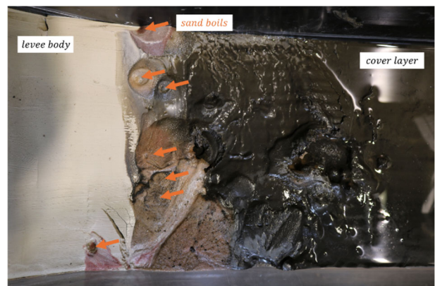
Figure 8. Geocentrifuge model (top view) with sand boils (indicated by orange arrows) located at the toe of the levee.
