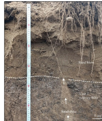
Figure 7. Example of sand dyke below its sand blow linked to the 2020 Petrinja earthquake ( Lat 45.471819°; Long 16.225298°)
