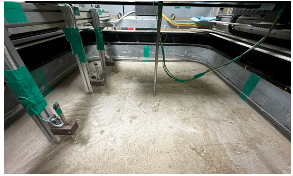
Figure 7. Centrifuge cone penetration tests carried out at KAIST.
