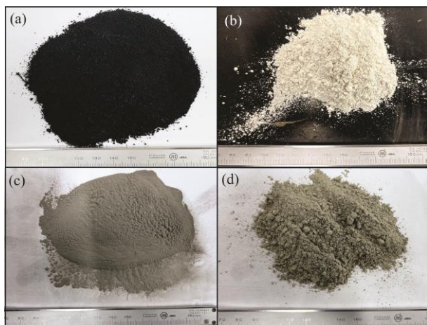
Figure 4. Additives (a) rCB, (b) hydrated lime, (c) cement, and (d) TB
