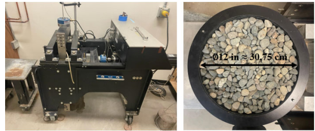
Figure 3. Large Scale Cyclic Simple Shear Device used for laboratory testing, University of California, Berkeley, GeoSystems Engineering Soil Mechanics Laboratory.
