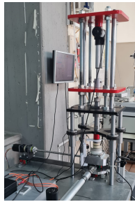
Figure 4. GeoAnts multi-directional cyclic direct simple shear (CDSS) apparatus.
