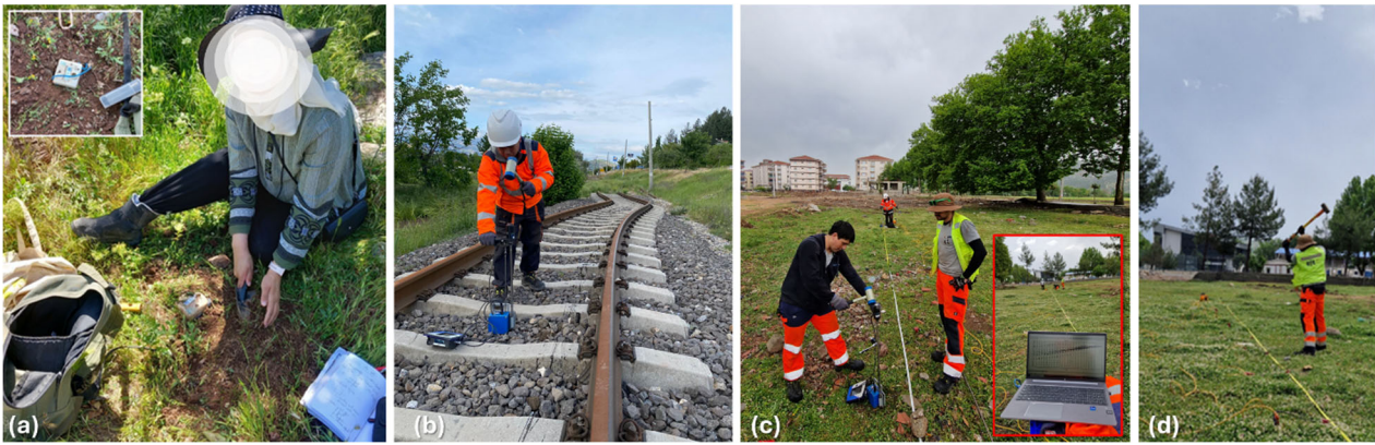
Figure 1. Illustration of portable geotechnical and geophysical test (a) HVSr, (b) iDCPT (Panda), (c-d) iDCPT (Panda) and 2DMASW measurements Illustrations of iDCPT (Panda®) and 2DMASW measurements carried out at Gölbaşı, (Türkiye) in May 2024.
