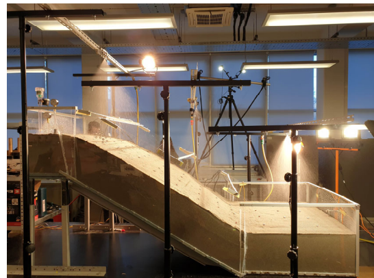
Figure 2. Z shaped experimental slope model inclined at 30^\circ .
