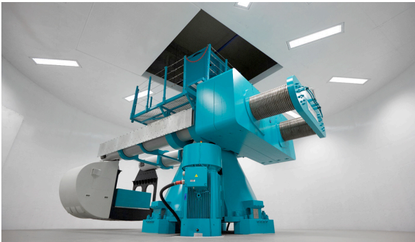
Figure 1. The 10 m diameter beam centrifuge at UWA
