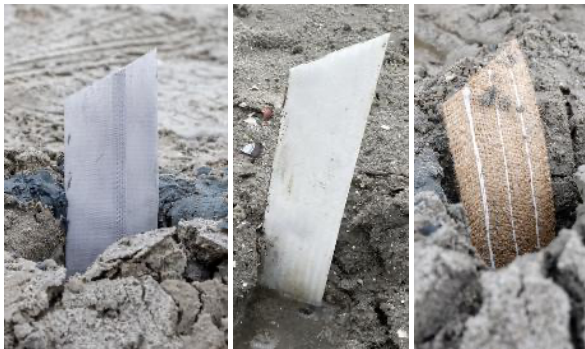
Figure 2. The trialed drain types. From left to right: MD7407, Biodrain and Green PVD.
