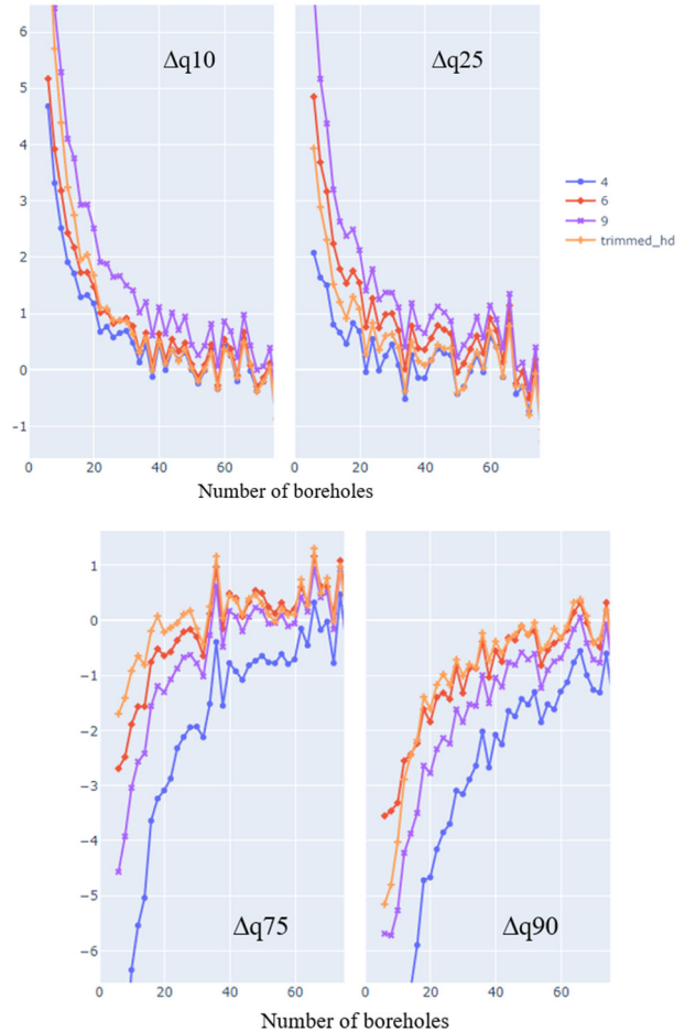
Figure 4. Global error as a function of the number of boreholes used to infer the quantile curves for 4 selected estimators
