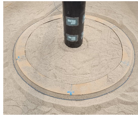
Figure 1. DFOS cable installation.
