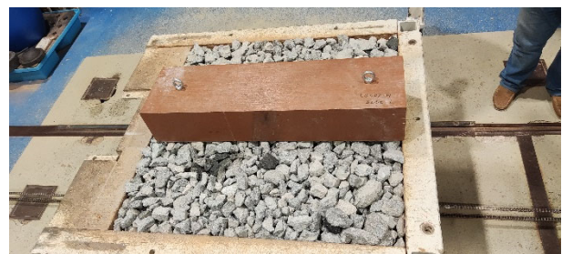
Figure 4 General aspect of the test set-up when concrete sleeper is used.
