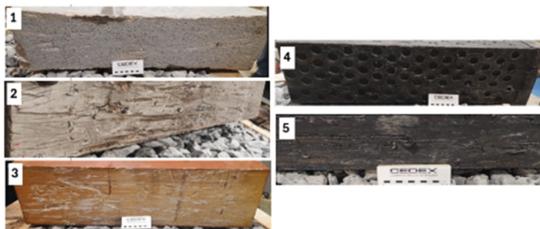
Figure 7 Aspect of the bottom of the sleepers after the tests.
