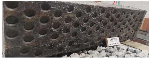
Figure 3 Detail of the base of the plastic sleeper.
