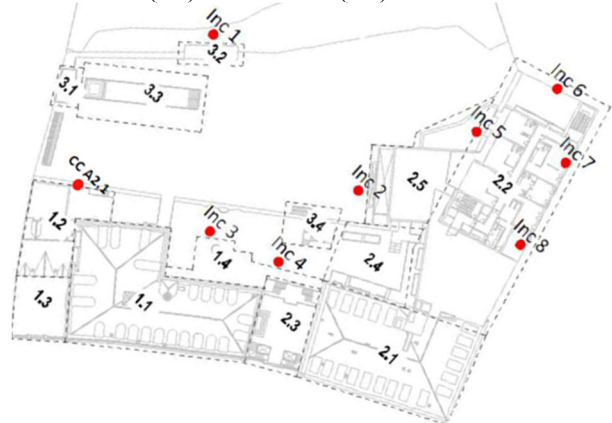
Figure 18. Inclinometers (Inc) and load cells locations (CC).
