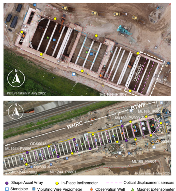
Figure 1. Site plan and instrument locations at BTEP (above) and BTWP and WHRC Section A (below).
