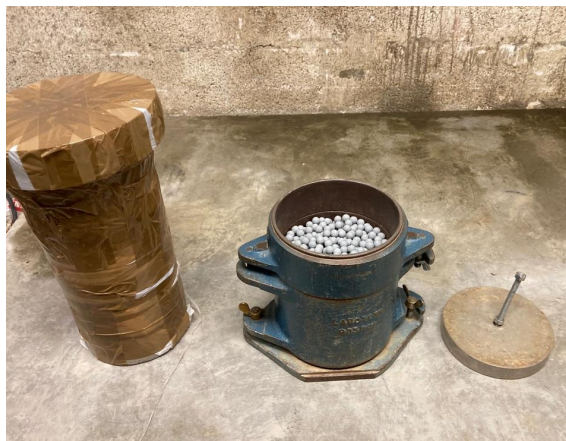
Figure 1. Mold with the grains and weight of 20 kg on the vibratory table to perform the measurements of e_{min} .
