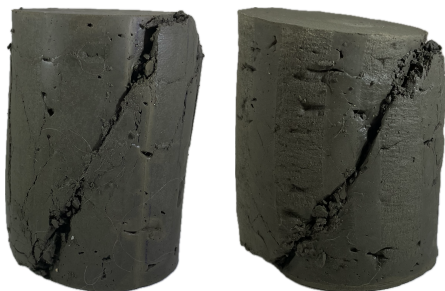
Figure 8. Failure mechanism. Left: ID 50; right: ID 8.
