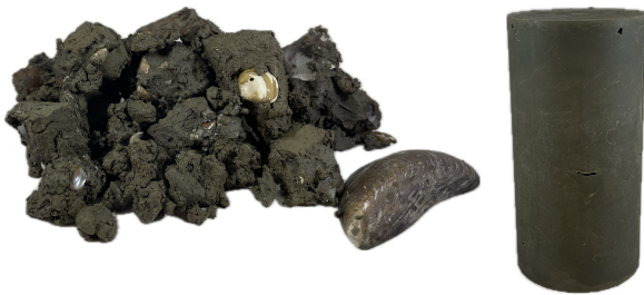
Figure 1. Left: natural gyttja; right: cement stabilized specimen.
