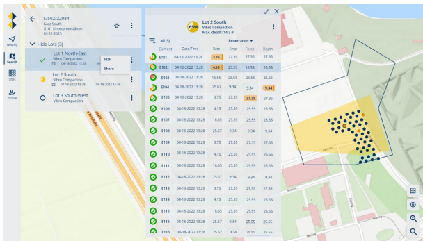
Figure 5. Screenshot of quality analysis application for project managers in the development phase
