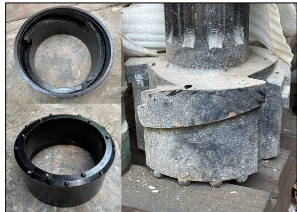
Figure 1. Sacrificial wing bit system: wing bit on the left, the driver and drill bit on the right.
