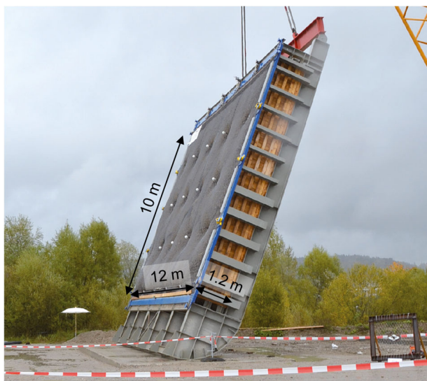
Figure 3. Test setup with the inclined steel frame.
