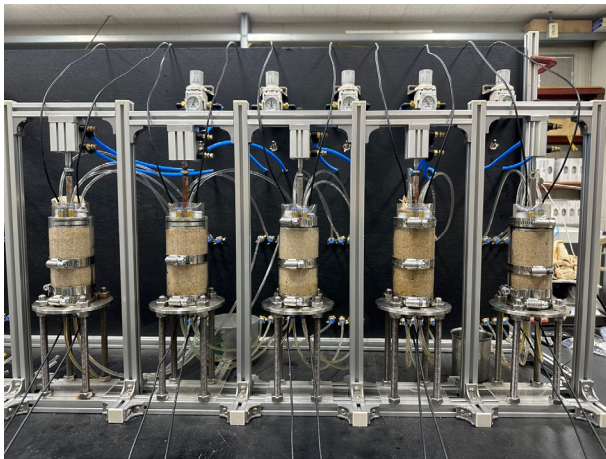
Figure 1. Test setup for bio-treatment and elastic wave measurements.
