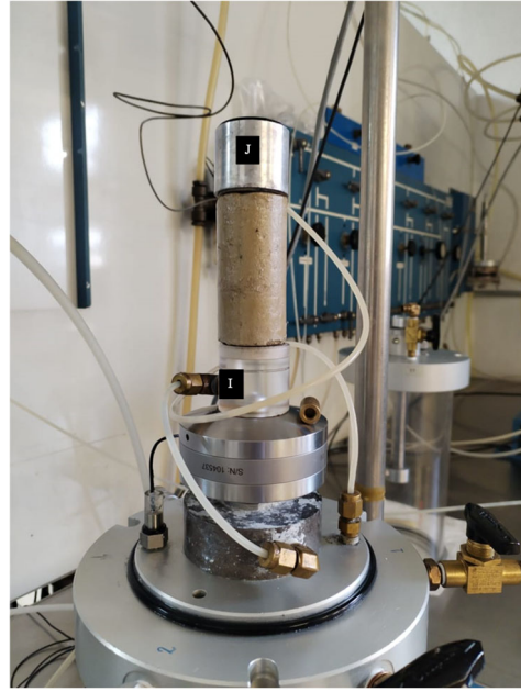
Figure 2. Pore pressure transducer at base and head of the specimen
