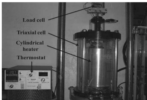
Figure 1. Suction and temperature controlled cyclic triaxial apparatus.
