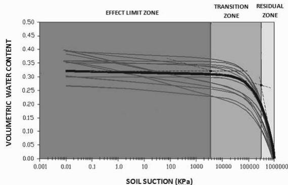
Figure 8. Typical SWCC for Clays (Type A).
