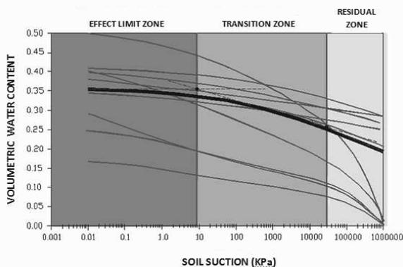
Figure 9. Typical SWCC for Clays-Limes (Type B).
