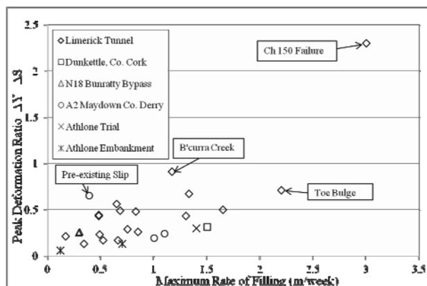
Figure 5 Peak Deformation Ratio v Max Filling Rate
