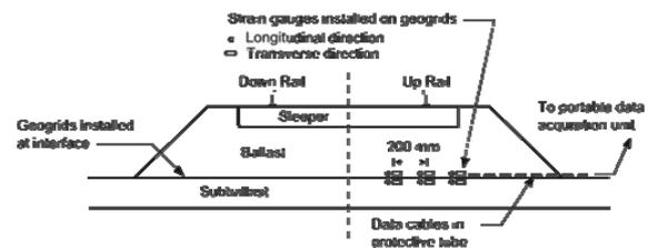
Figure 5. Details of track instrumentation using strain gauges.
