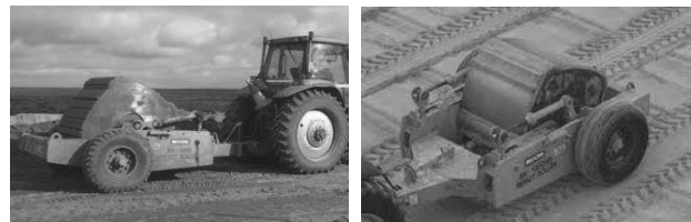
Figure 1. An example of RDC – Broons BH-1300 4-sided impact roller.
