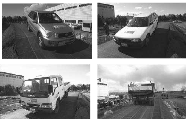
Photographs 8. Trafficability tests of Confined-Reinforced Earth
